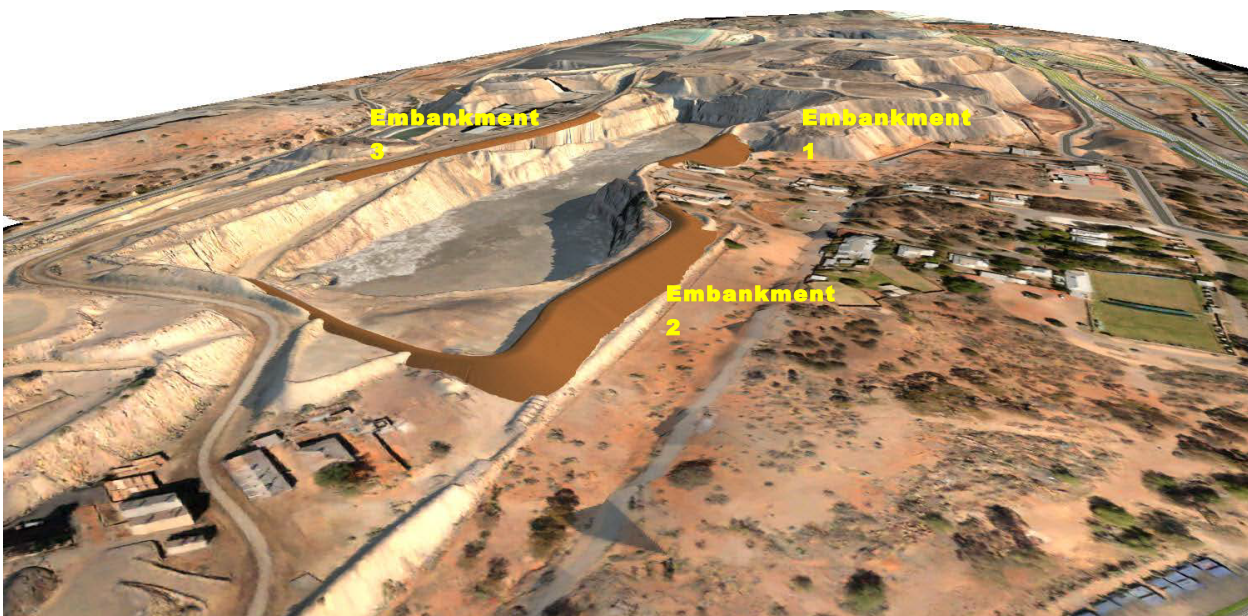
Figure 10-14 Impression of Embankments
