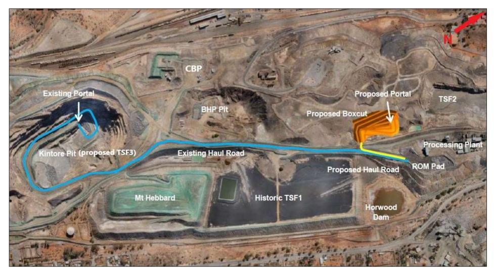
Figure 2.1 Indicative site layout showing the proposed new portal, boxcut, TSF2 and TSF3
