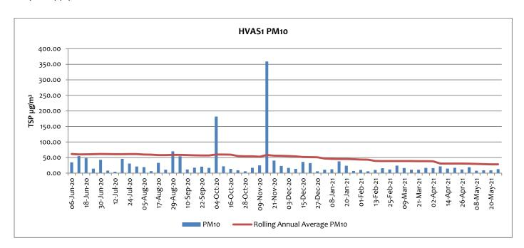
$PM_{10}$  dust results at HVAS1 were low for the month of May. The annual rolling average for  $PM_{10}$  dust at this location is 28.2  $\mu g/m^3$  at the end of May 2021, lower than the average at the beginning of June 2020 which was 61.4  $\mu g/m^3$ . External dust events are recorded in measurements.
