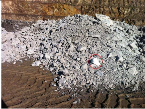
Photo 1: Part of the waste rock stockpile showing hard hat for rock size reference
