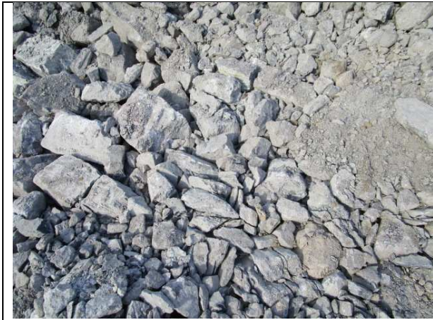
Photo 7: Close up view of waste rock material, note: large degree of variation in sizes
