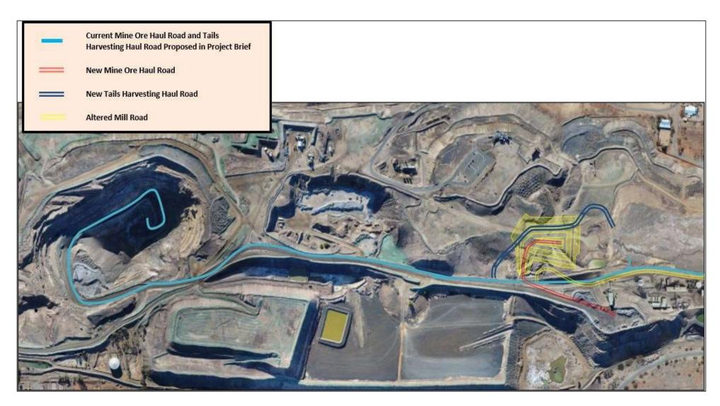
Figure 2.1 Current mine haul roads and proposed new tailings harvesting haul road
