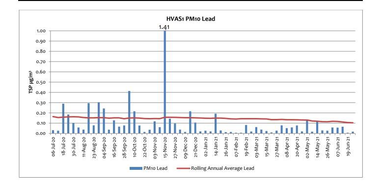
$PM_{10}$  lead levels were low in June 2021. The rolling annual average for  $PM_{10}$  Lead in June 2021 was 0.11 µg/m<sup>3</sup>, down from 0.16 µg/m<sup>3</sup> in July 2020.
