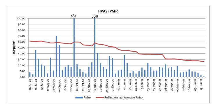
$PM_{10}$  dust results at HVAS1 were low in the month of June. The annual rolling average for  $PM_{10}$  dust at this location is 26.3  $\mu$ g/m<sup>3</sup> at the end of June 2021, significantly lower than the average at the beginning of July 2020 which was 61.2  $\mu$ g/m<sup>3</sup>. External dust events are recorded in measurements.
