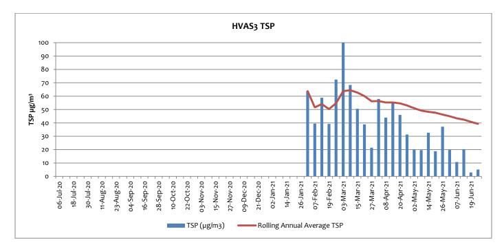
The rolling annual average for TSP Lead in June 2021 was 0.32  $\mu$ g/m<sup>3</sup>, however due to the unit being reinstalled after 19 months decommissioned, annual rolling average is calculated using data from February to June only.
