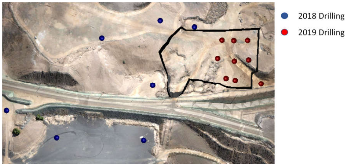
Figure 5 Plan view of diamond drill investigation holes
