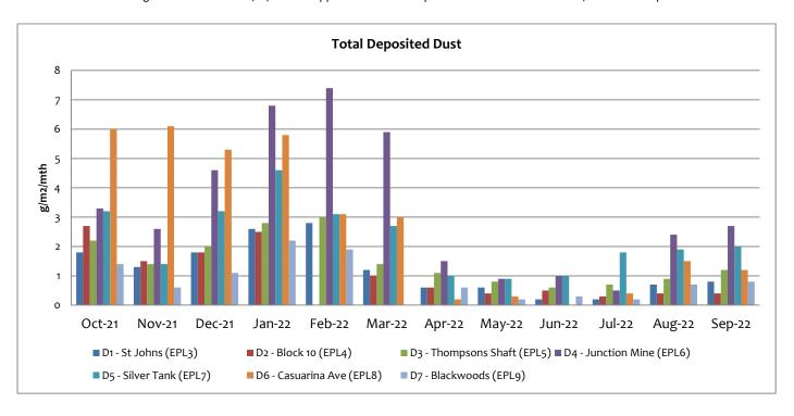
The dust levels recorded in Dust Gauges in September 2022 were consistent with previous months. The highest dust levels were recorded in the D4 Junction Mine gauge. The predominant wind direction for September was from the South as shown in the Wind Rose in Section 4, suggesting there may have been contribution of dust from sources on-site such as the rail loadout, Blackwood's waste dump and TSF.
