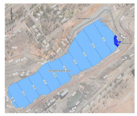
Figure 2: Stage 1 Intermediate Tailing Deposition
