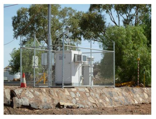
Photo 2. Automatic air quality monitoring station, dust deposition monitor and noise monitor.
