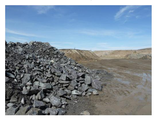
Photo 16. ROM pad showing ore stockpile, bunds and water sprays.
