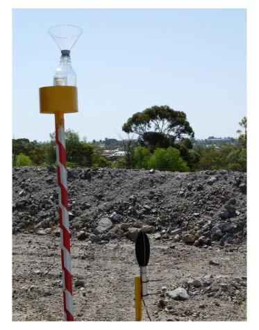
Photo 28. Dust sampling jar on site and microphone for noise monitoring.
