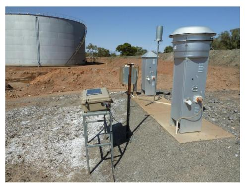
Photo 1. Automatic air monitoring station, noise and vibration monitors.
