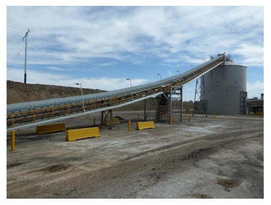
Photo 7. Covered conveyor from crusher to ore storage bin.
