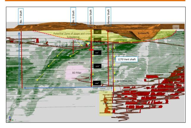
Figure 10- Zone of potential subsidence down to 525' level underneath Kintore Pit (looking west)
