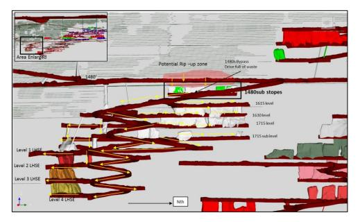
Figure 20- Pathways associated with ingress from the 1480sub stopes to LHS and LHSE.
