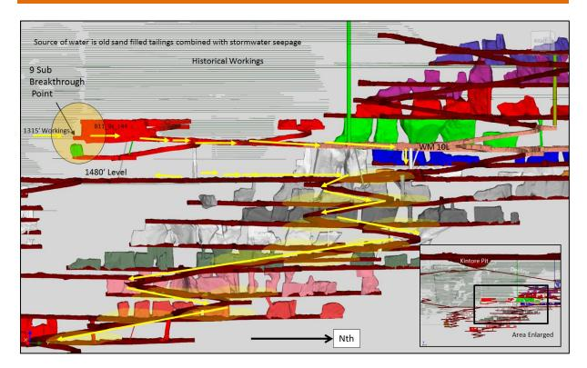
Figure 18- Potential WM fluid pathway from 9sub and connection with the 1315 ft workings
