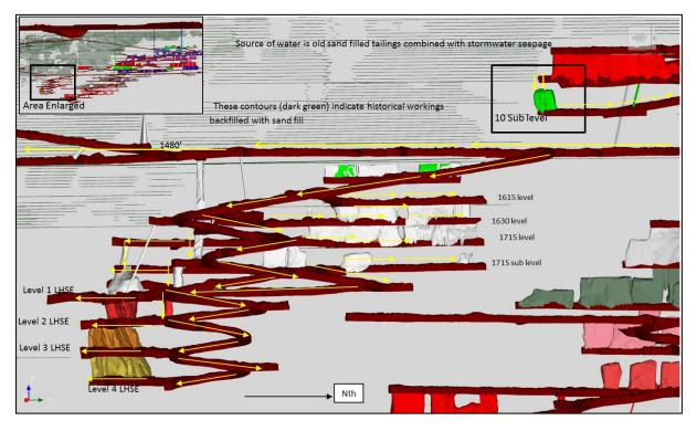
Figure 21- Block 11 10sub stope illustrating fluid connectivity with the 9sub failed stopes.
