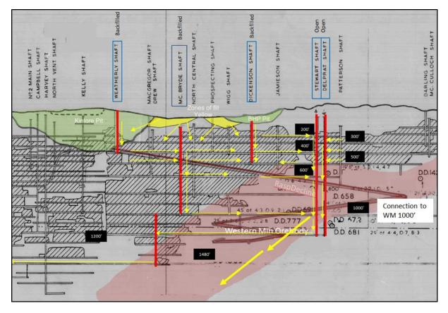
Figure 15- Potential pathways for Weatherly, McBryde Shaft, Dickenson Shaft, Stewart Shaft and Delprat Shaft
