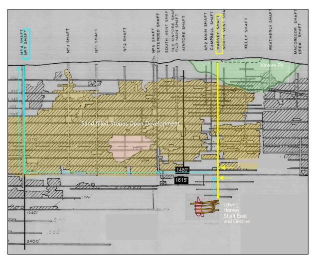
Figure 7- Harvey shaft cross section potential fluid pathway
