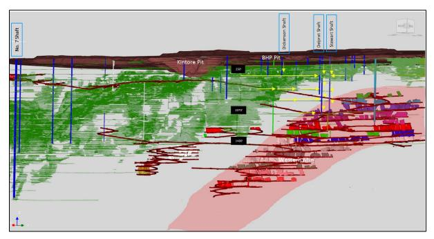
Figure 16- Potential fluid pathways for the Dickenson Shaft, Stewart Shaft and Delprat Shaft
