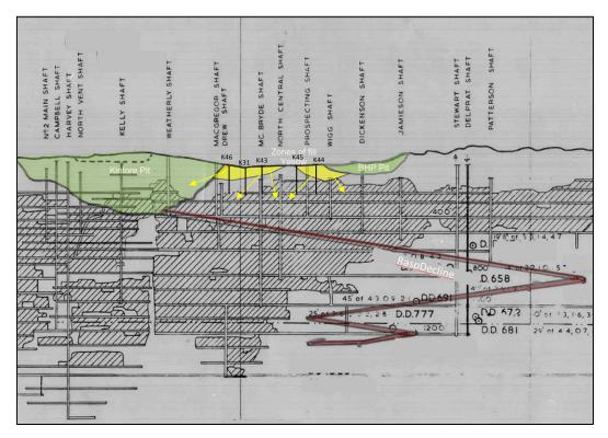
Figure 12- Potential fluid pathway related to historical fill between the BHP Pit and Kintore Pit. Note the 5 percussion drill holes drilled by MMM (locations approximate)
