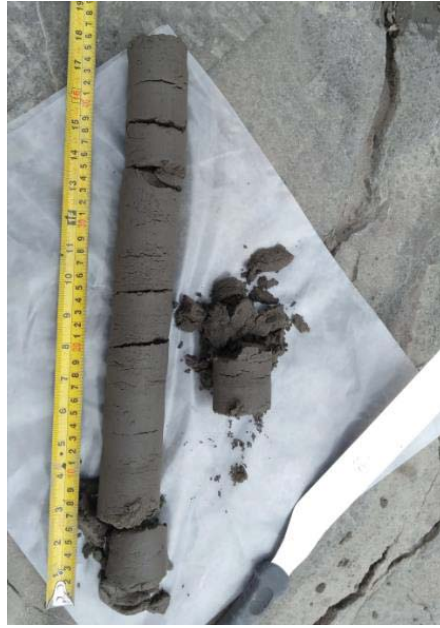
Figure 3 Sample Ready to Divide Into 100mm Increments
