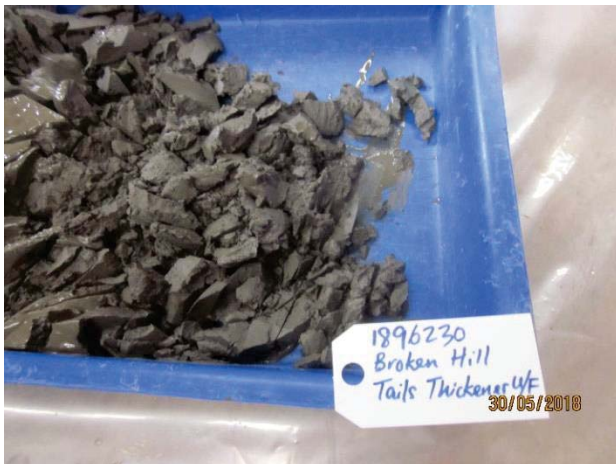
Figure 2: Material transferred to plastic container for drying at 50°C
