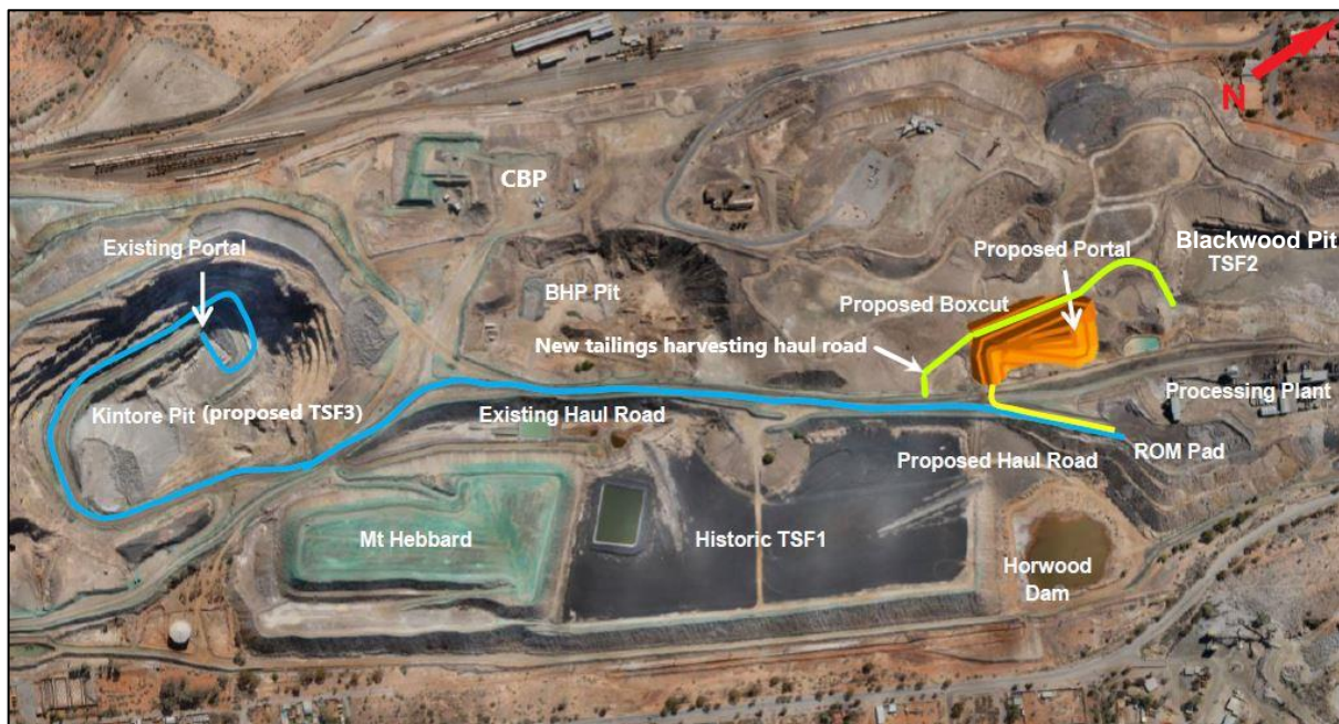
Figure 1: Tailings and Waste Rock Management Layout
