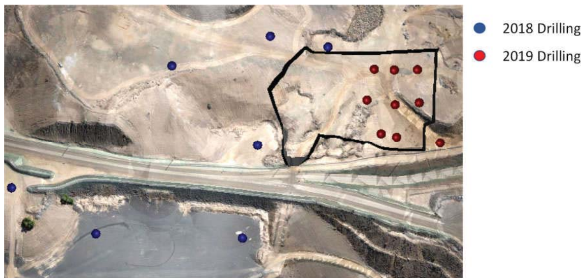
Figure 5 Plan view of diamond drill investigation holes
