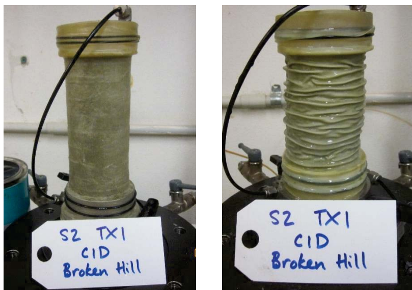
Figure 3: Example of specimen before and after triaxial test
