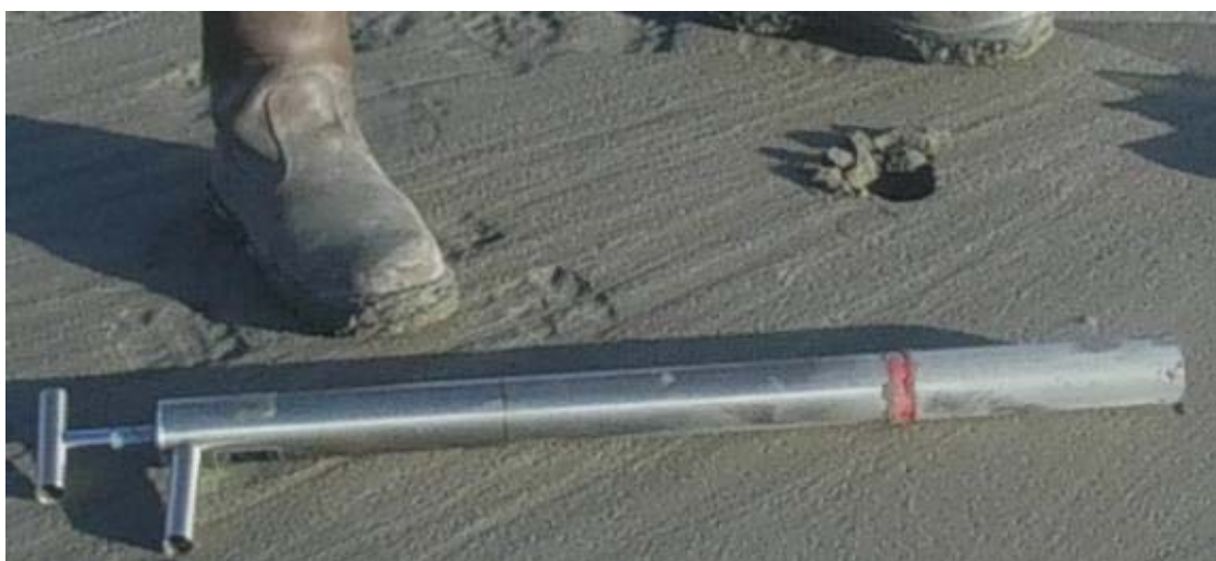
Figure 2 'Yabby Pump' sampling device with remaining hole
