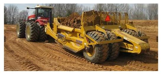
Figure 5-1: Example of rubber tyred tractor scoops proposed for tails harvesting
