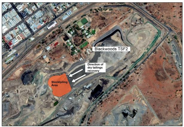
Figure 2-1: Indicative locations of stockpiling and dry stacking
