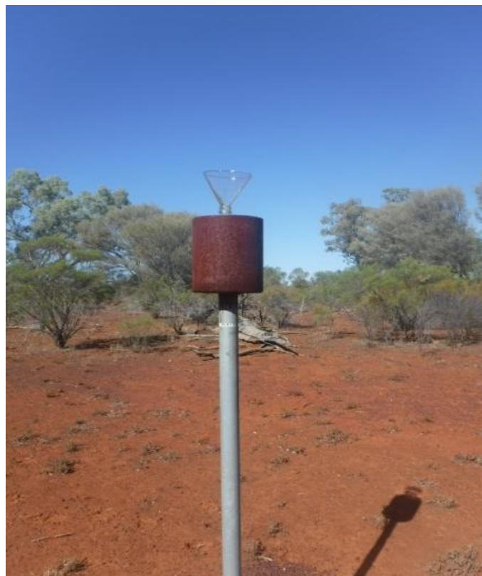
Figure 3.1 Dust monitoring gauge located in the project
