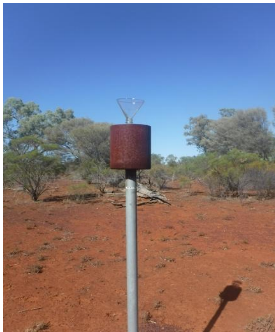
Figure 2.1 Dust monitoring gauge located in the project
