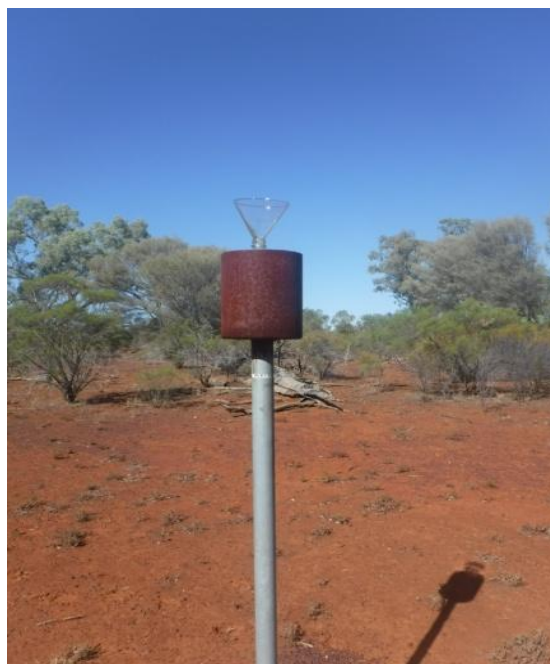
Figure 2.1 Dust monitoring gauge located in the project
