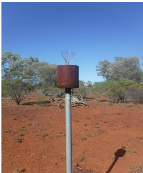
Figure 2.1 Dust monitoring gauge located in the project
