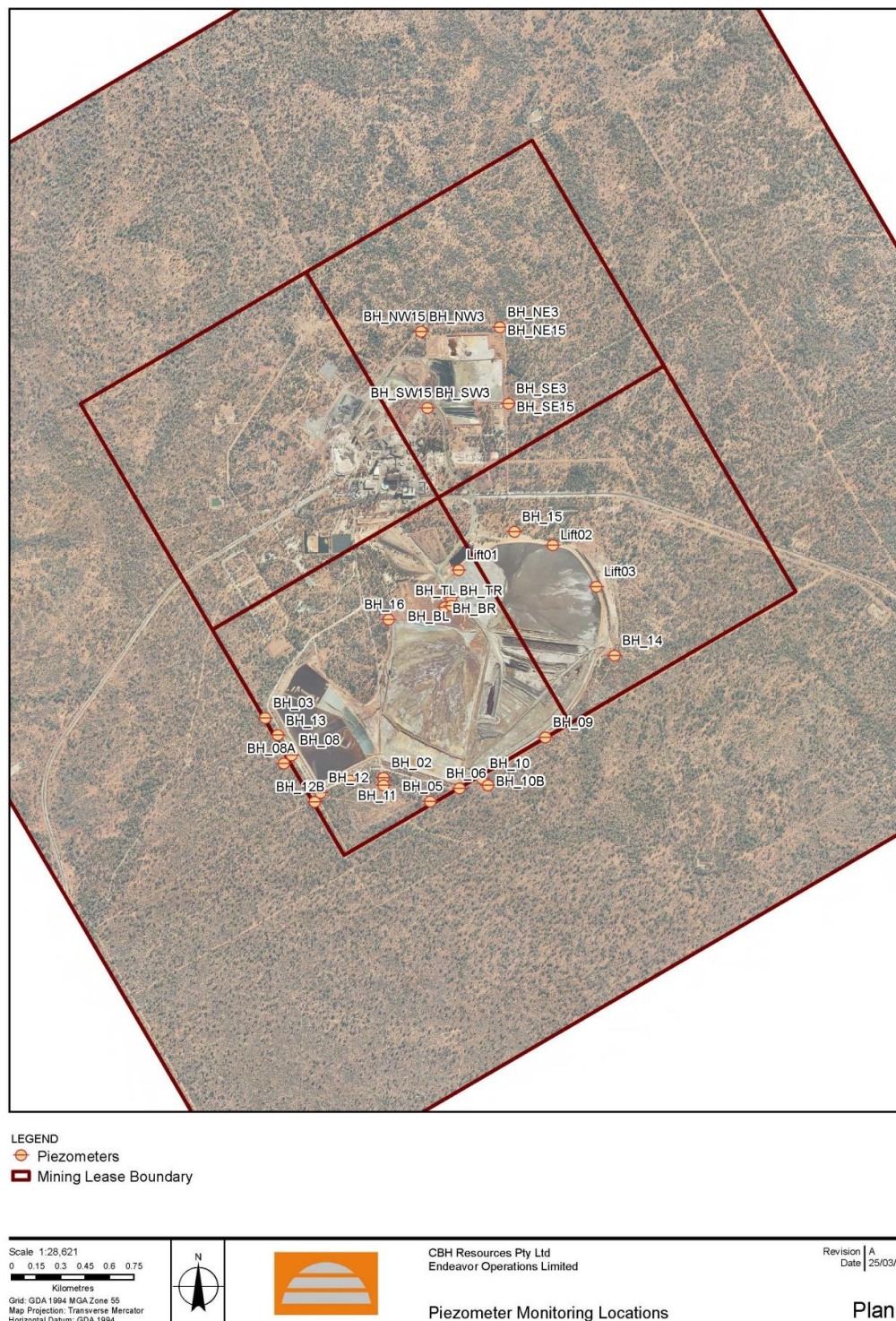
Figure 2.3 Location of the Piezometer Monitoring Locations
