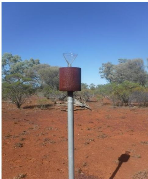
Figure 2.1 Dust monitoring gauge located in the project
